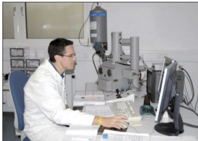
The high-tech equipment for quality control of the VITA laboratories also includes a scanning electron microscope.
