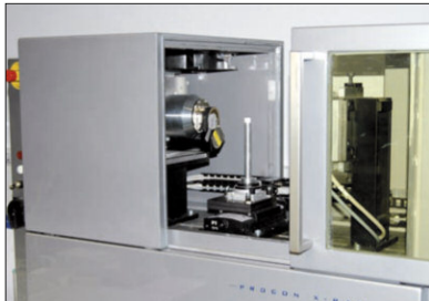
Cracks in the material structure of CAD/CAM blanks can be detected in a computer tomograph.
