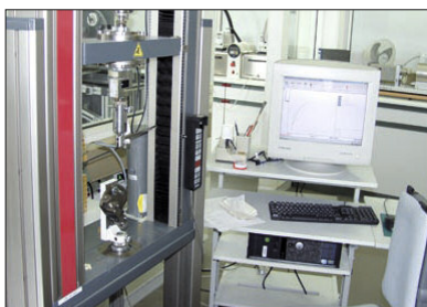
Universal testing machine for the 3-point bending test (photo source: DIGITAL_DENTAL_NEWS)
